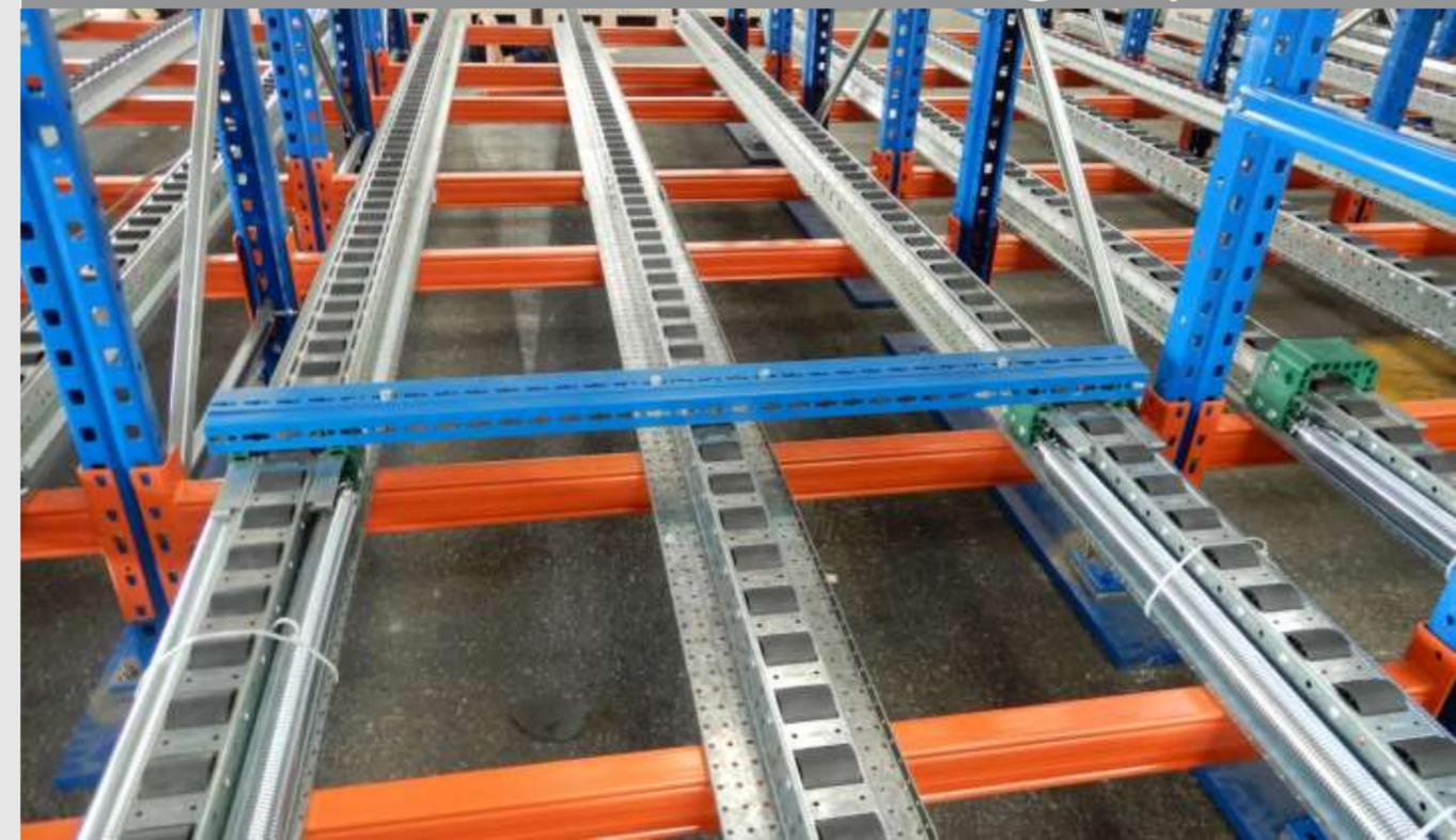
Added central roller track provides additional support to weak pallet
